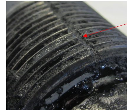
Blocked equalization channel on a hollow carrier plug
