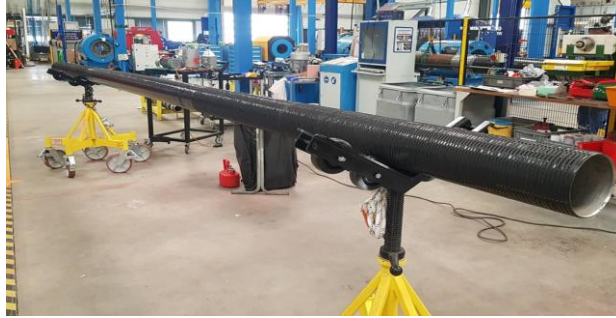
Figure 4-Expandable Tubing Patch with fully covered elastomer
