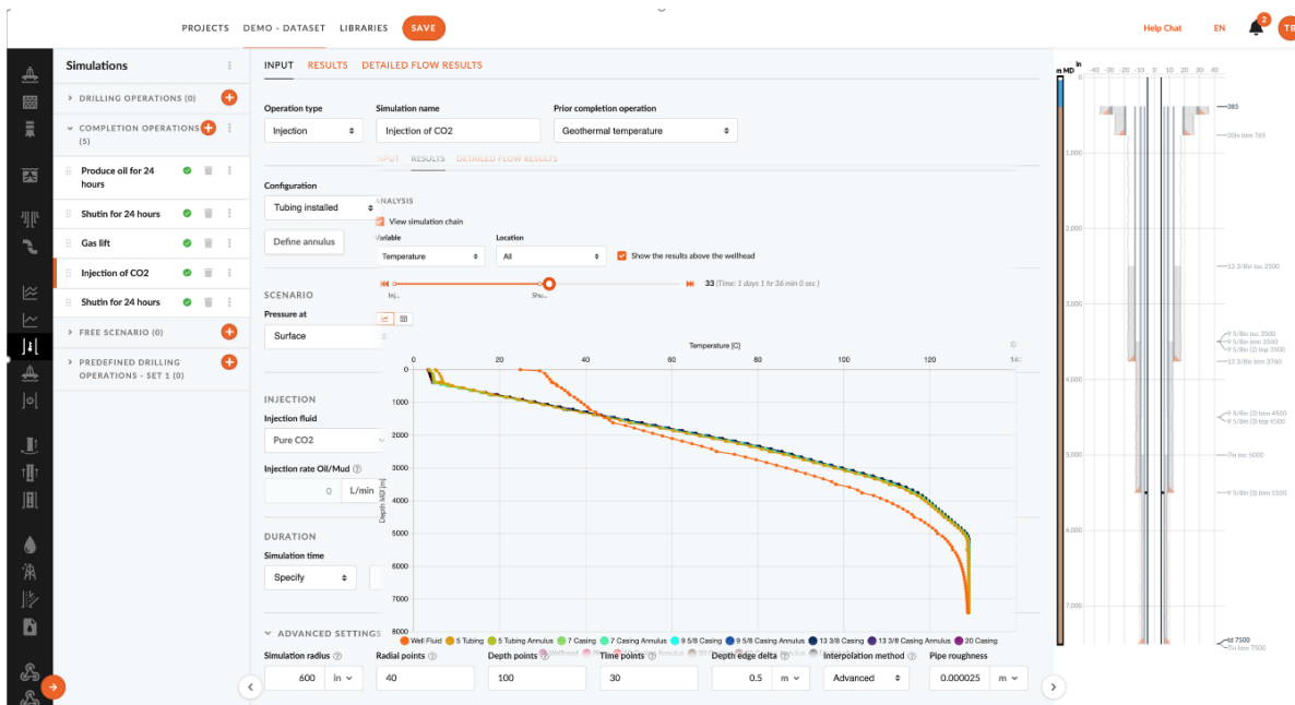
Fig.2: Example of Thermal Simulations for Liquid CO2 Injection
