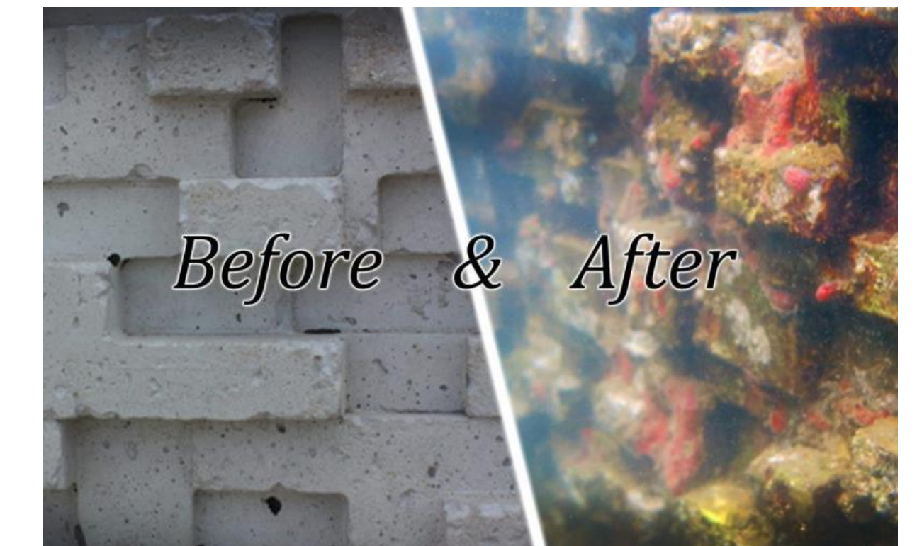
Fig 3: Eco-concrete before and after to show how marine life thrives when used. 80% less carbon footprint
