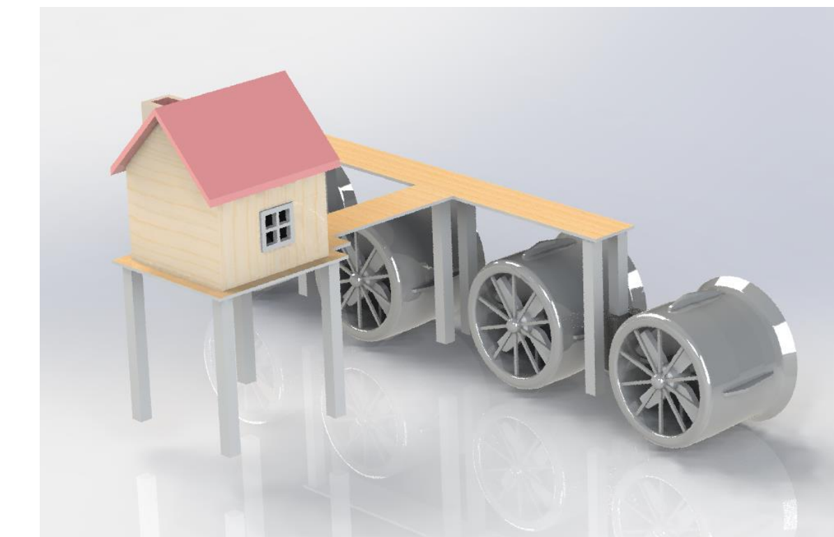
Fig 2: Extend working pier or extension of seawall so as to reach 20-30 m depth. Vertical alignment of turbines
