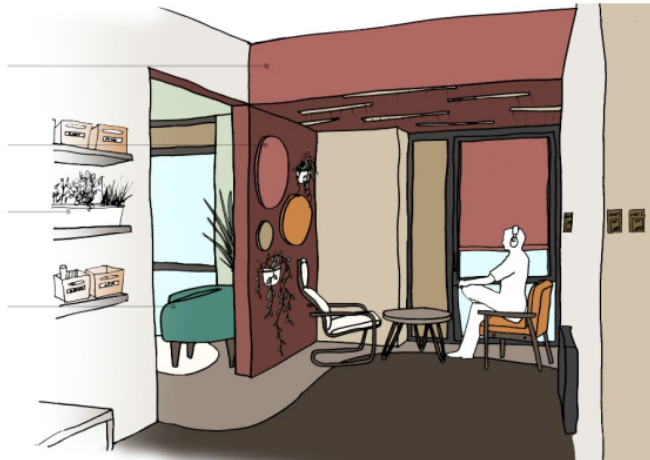
EXAMPLE OF A TRANSITION SPACE WITH VARIATION OF CEILING HEIGHT TO CONCEAL MVHR UNITS
