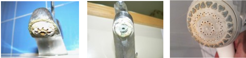
Fig. 5.3.5. Scale formation on taps and shower head
