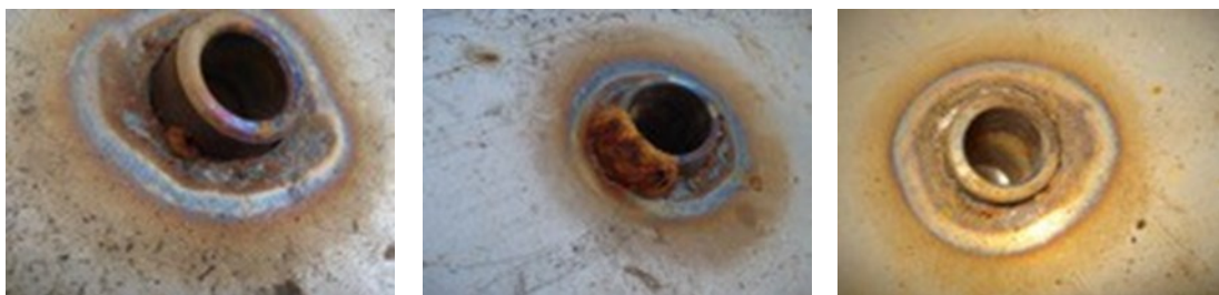
Fig. 5.1.1 Failed welds in stainless steel tanks
