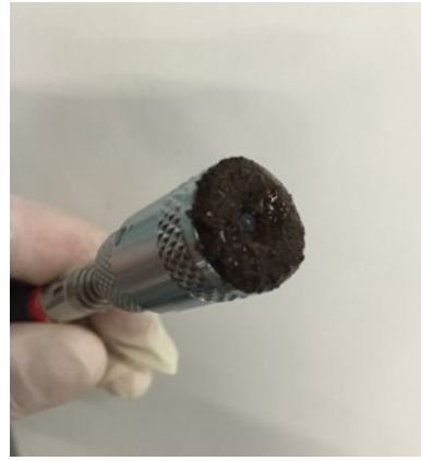
Figure A6.1.2: System Iron Oxide on Magnet
