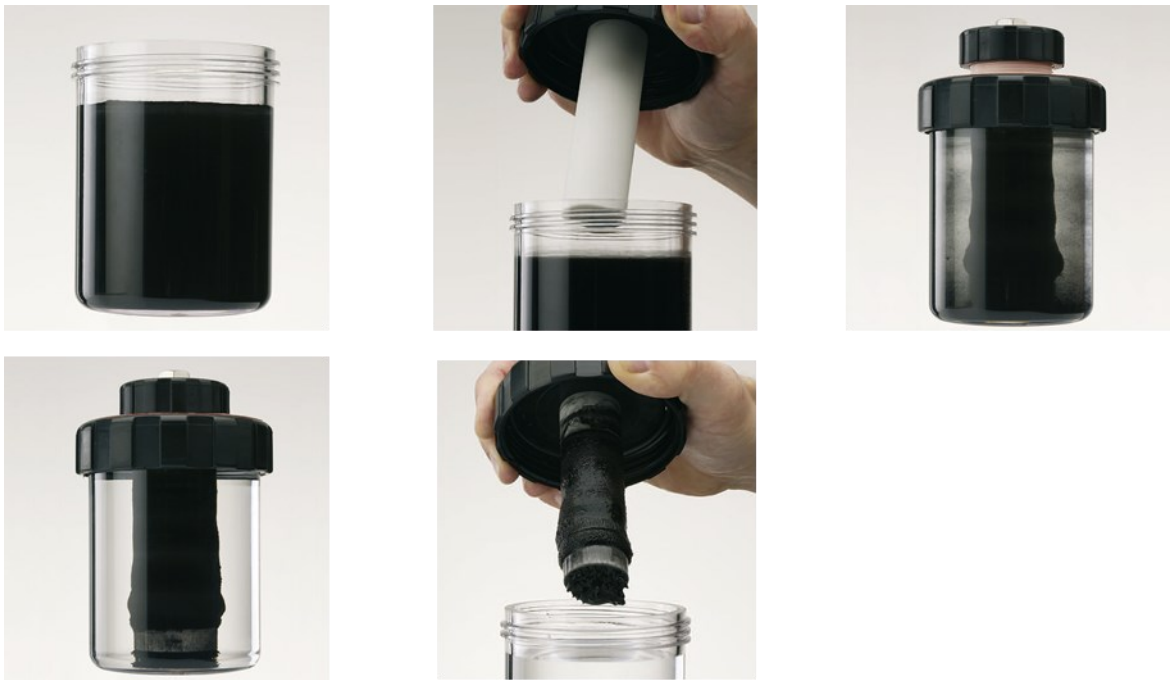
Figure A6.3.1: Demonstration of Magnet Effect on Magnetite
