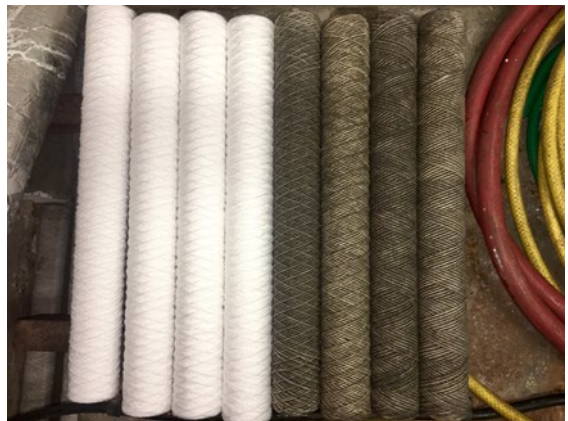
Figure A6.2.2: Sludge Contaminated (new/old) Filter Cartridge
