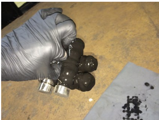
Figure 5.5.1: Contamination by High Levels of Suspended Solids
