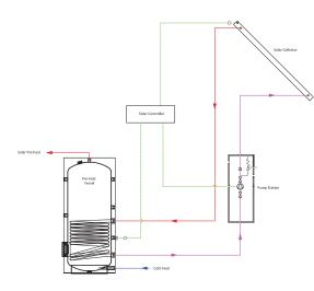
Indirect water heater operating as pre-heat vessel with solar thermal
