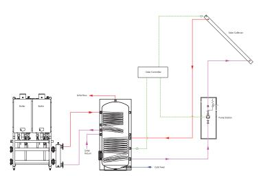
Twin coil indirect water heater with solar thermal and gas-fired condensing boilers
