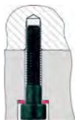
2) Individual base plate securely bolted to housing from below through all 4 holes
