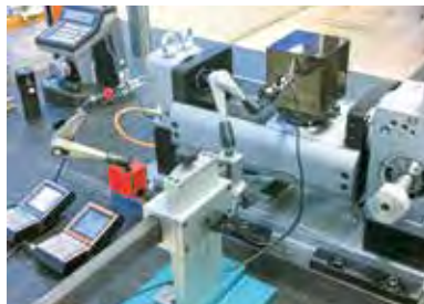
Measuring a T-type rotary table with a cube
