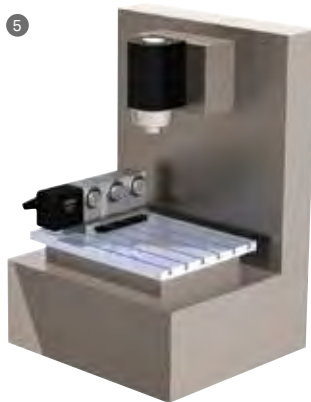
5 4th axis, 3-spindle, Y-mounting (crosswise)
