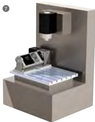
7 4th + 5th axis, 2-spindle, Y-mounting (crosswise)
