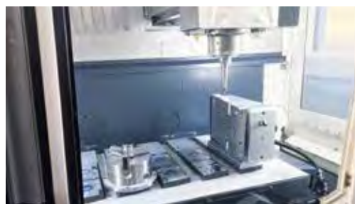
Application of a 4th axis on a 3-axis machining center
