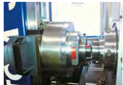
Measuring the indexing accuracy - fully automatically
