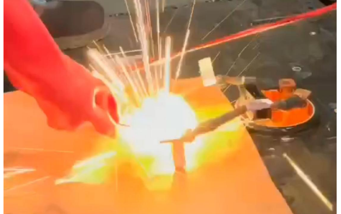
Illustrative example of a short-circuit error on a battery pack (Source: Duesenfeld GmbH)
