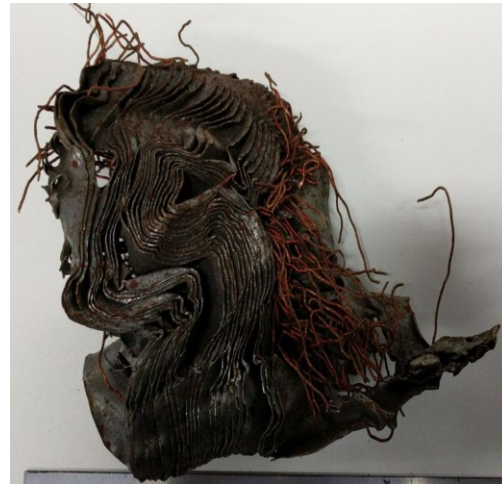
Shredded automotive motor (courtesy of Axion)
