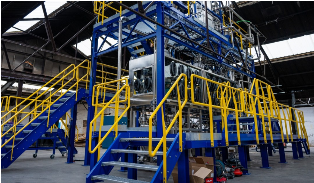
Automated powder processing – Sieving, jet milling, blending
